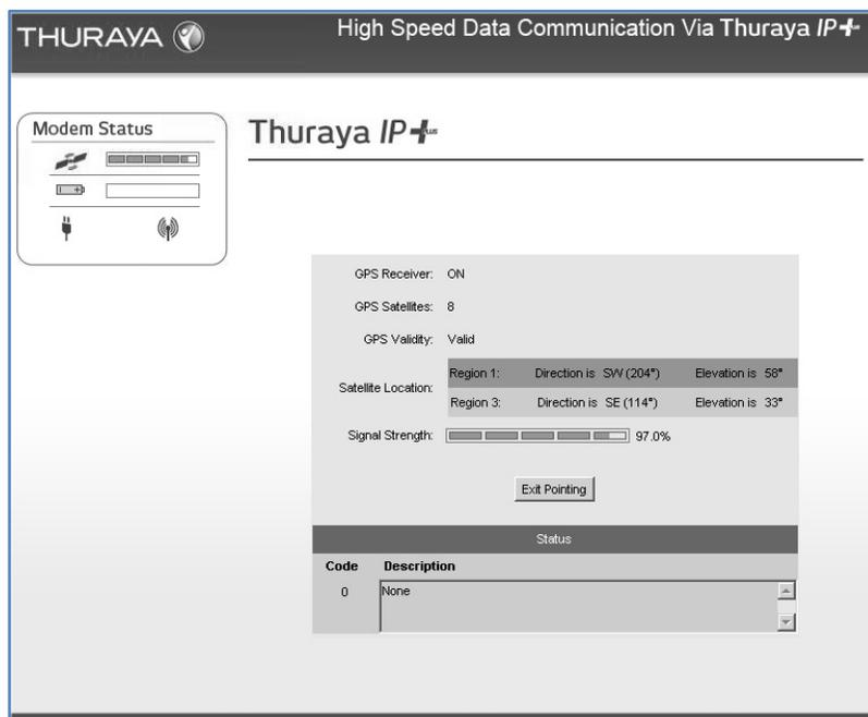
The **Antenna Pointing Screen** step can be enabled using the **Antenna Pointing** option on advanced settings screen described above. When this option is **enabled**, the Thuraya IP+ will stop in a pointing mode prior to accessing the network after powering up. This can be useful when optimal pointing is important, such as with fixed installations using an external antenna.
