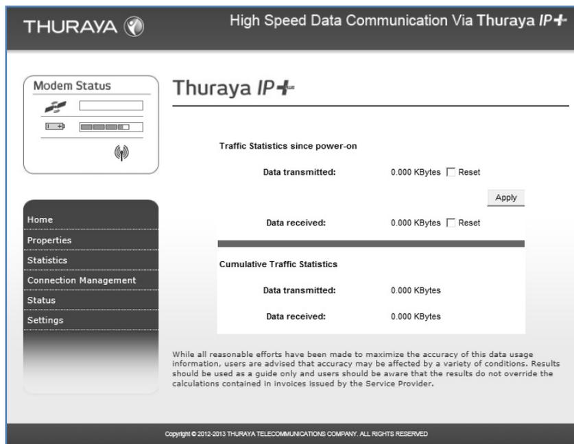
The **Statistics Screen** provides you with an estimate of your data usage. Data usage figures are obtained by counting the bytes in the IP packets received by and sent from the Thuraya IP+ terminal. You can view both “since power on” (per session) and “Cumulative” (lifetime) data usage counts. To reset the data counters of a session, simply select the **reset** button for either transmit or receive and click the **Apply** button.
