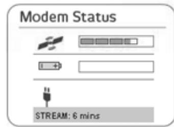
There is also a streaming timer embedded within the Modem Status box that appears on the upper left hand corner of the web page. This provides an indication of how long the streaming session has been active.
