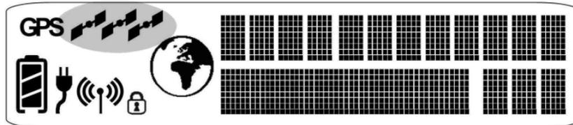
When the **GPS** icon stops flashing then Thuraya IP+ has successfully updated its GPS position.
