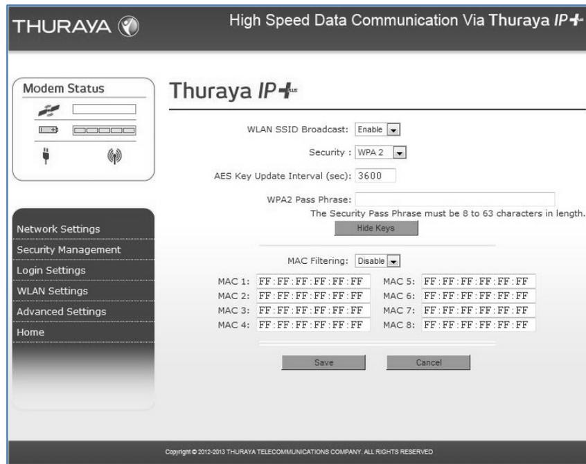
The **WLAN Security Screen** allows you to configure WLAN security parameters, including enabling/disabling Wired Equivalent Privacy (WEP), hiding the SSID and setting Media Access Control (MAC) filters.
