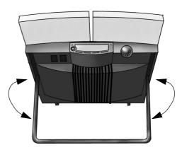
Tilt the EXPLORER 500 slowly up or down until it points in the correct vertical direction, known as the **Elevation**.
