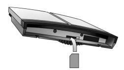
3. Slide the lock to close the SIM slot.
